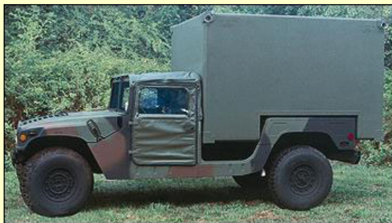
The S-788 shelter, also known as the Lightweight, Multipurpose Shelter (LMS) is a lightweight, high strength enclosure designed specifically for use on the HMMWV. The S-788 provides approximately 295 cubic feet of useable interior space and weighs only 608 pounds, allowing it to be transported easily on C-130. The U.S. Army uses the S-788 as its primary electronics platform for wheeled tactical vehicles.
